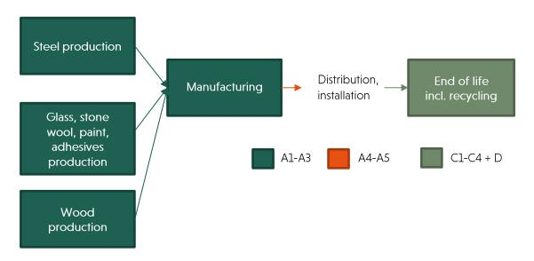
Materials such as galvanized steel, coated galvanized steel, stone wool, paint, adhesives, silicon, and glass are transported to the manufacturing plant (Daloc AB), where the steel doors are manufactured. The wood used as threshold comes to Daloc AB from the wooden doors manufacturing site (Daloc Trädörrar AB). From the manufacturing site, the doors are transported to the customers. After use the product is
